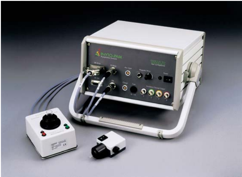
Fig. 3 Emitter-Detector Unit PHYTO-ED (left) with Stirring Device WATER-S (right) and Power-and Control-Unit PHYTO-C
