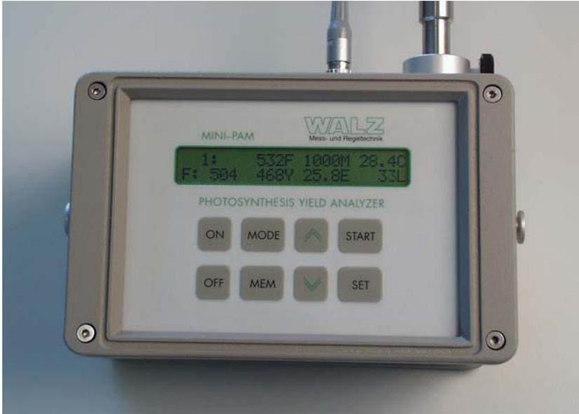
Fig. 1: Photosynthesis Yield Analyzer MINI-PAM
