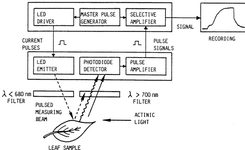
Fig. 11: Schematic view of the PAM measuring principle
