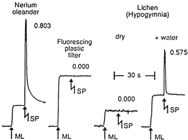
Fig. 12: Comparison of fluorescence responses of photosynthetically active (Nerium; Lichen, +water) and inactive (Lichen, dry) plant samples with those of a fluorescing plastic filter. ML, measuring light; SP, saturation pulse. The calculated values of effective quantum yield of energy conversion in PSII (YIELD) are depicted.
