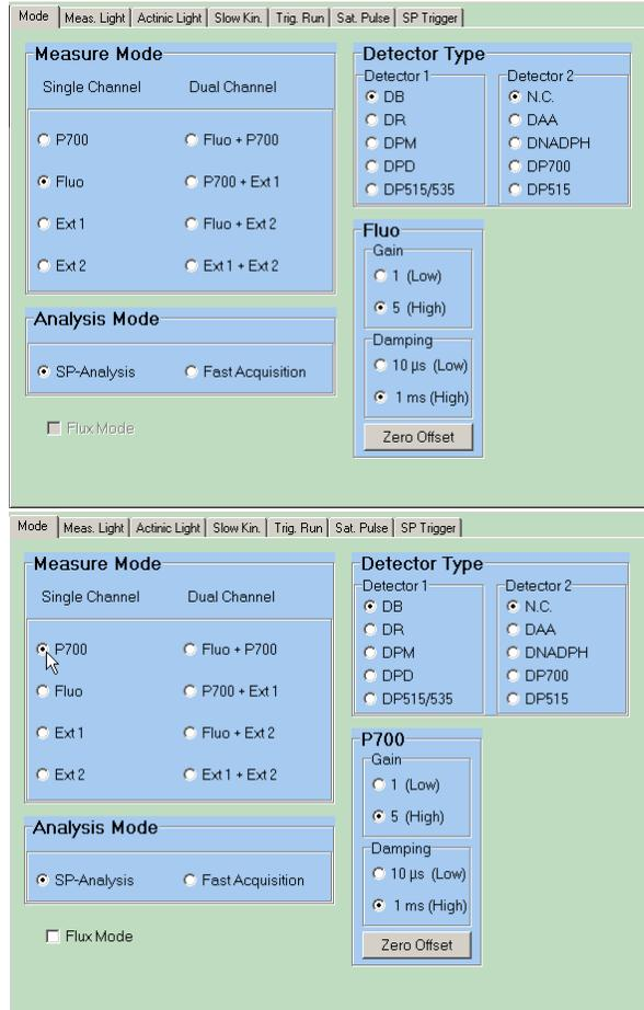
Fig. 8 Settings Measure Mode; top: Chlorophyll fluorescence; below: P700 measurement
