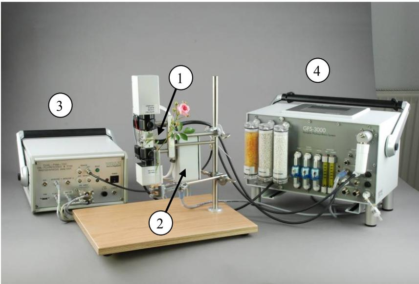
Fig. 1 Overview: Dual-PAM Cuvette (1) with Electronics Box (2), Dual-PAM (3) and GFS-3000 Central Unit (4).
