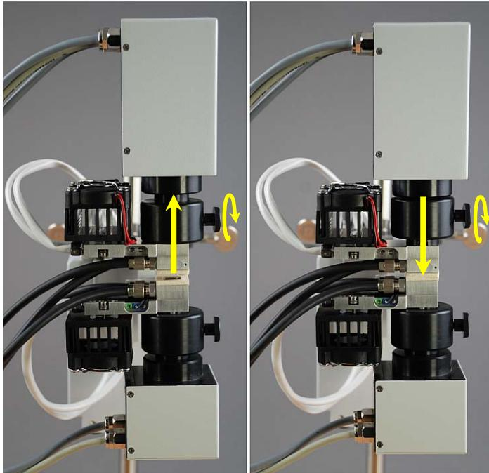
Fig. 4 Opening and closing of the cuvette
