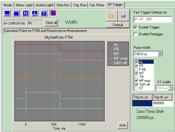
Fig. 22 Saturation Pulse triggering schedule for Induction Curve recording in the Dual Channel mode
