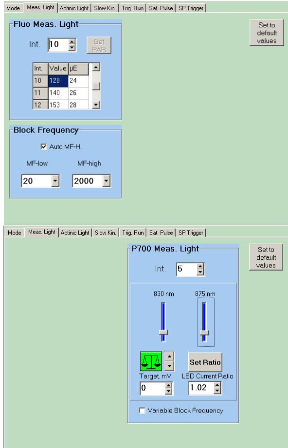
Fig. 9 Settings Measuring Light; top: Chlorophyll fluorescence; below: P700 measurement
