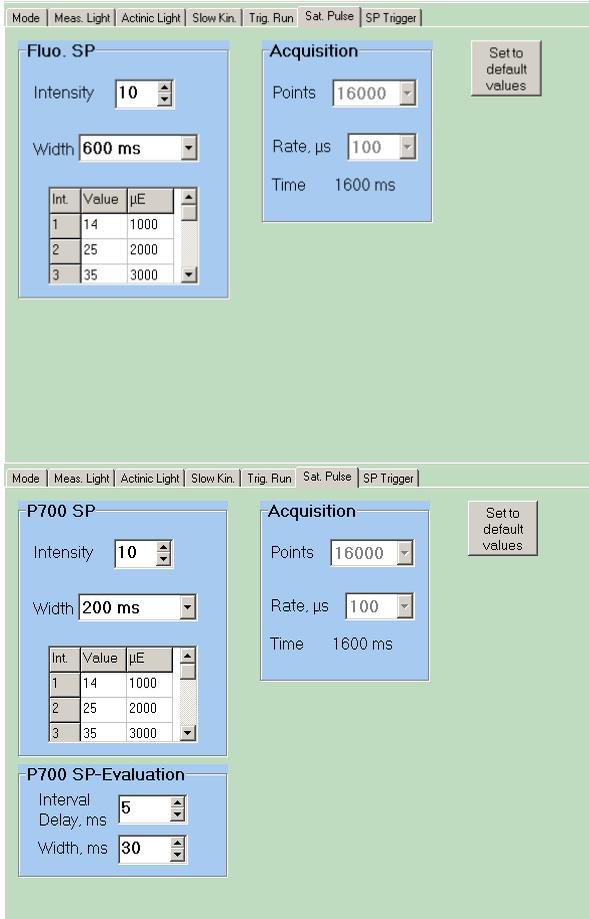
Fig. 10 Settings Saturation Pulse; top: Chlorophyll fluorescence, below: P700 measurement
