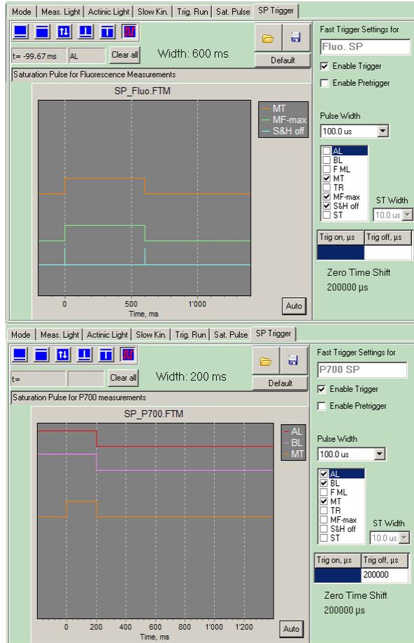
Fig. 11 Trigger Schedule for Saturation Pulse; top chart: Chlorophyll fluorescence; chart below: P700 measurement
