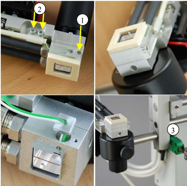
Fig. 30 Exchange of thermocouple
