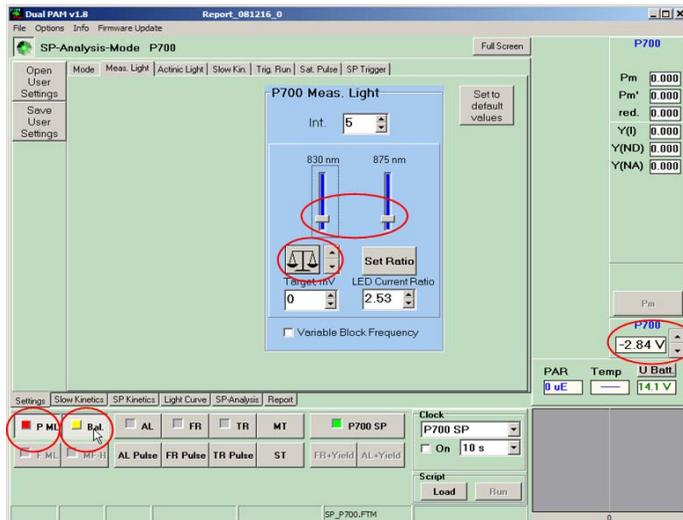
Fig. 15 Balancing of the P700 Measuring Light
